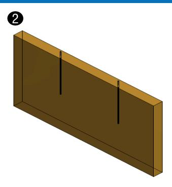
1.1.- Place the wall shoe inside the mould and pour concrete making sure that it does not enter in the wall shoe.
