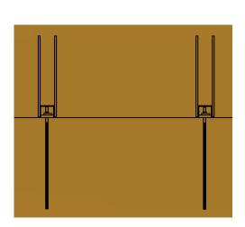
3.1.- Bring the panel closer to the foundation or to another panel and insert the wall shoe PPR into the anchor bolt TN. Once inserted, fix the conection with the squared washer and the screw
