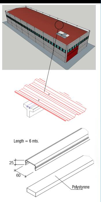
Anchorage for fixing sheet metal roofs on a prefabricated concrete element. Assembly using self-tapping screws.
