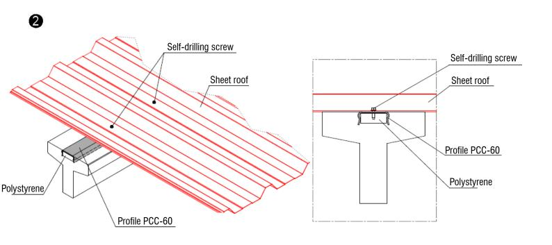
2.1.- Final check and assurance of tightening of self-tapping screws.
