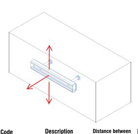
CodeDescriptionDistance between connectorsHPN240RProfile NOXI R length 24 cm160 mm55 mmPN240R-P35Profile NOXI R length 24 cm160 mm35 mm
