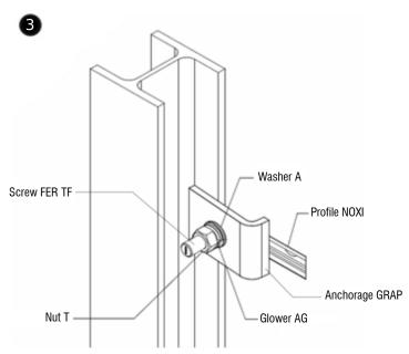
3.1.- Tighten the nut to finish the assembly. The Glower washer should be completely flat.
