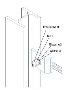
CodeDescriptionØ HoleGRAP17Anchor for retaining concrete panels with the<br/>steel structure using screws M16.17mmGRAP13Anchor for retaining concrete panels with the<br/>steel structure using screws M12.13mm
