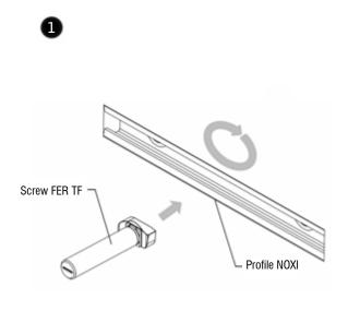
1.1.- Place the FER TF screws into the profiles\* and turn it 90 degrees.
