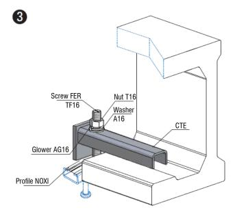
3.1.-Tighten the nut to finish the assembly. The Glower washer should be completely flat.3.2.- Final check and assurance of nut tightening.
