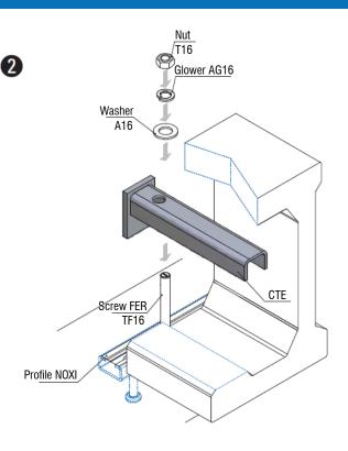
2.1.- Assembly of the screw and the CTE anchorage through the  $\emptyset17$  hole.
