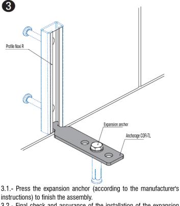
3.2.- Final check and assurance of the installation of the expansion anchor.
