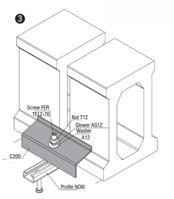
3.1.- Tighten the nut to finish the assembly. The Grower washer should be left completely flat.
