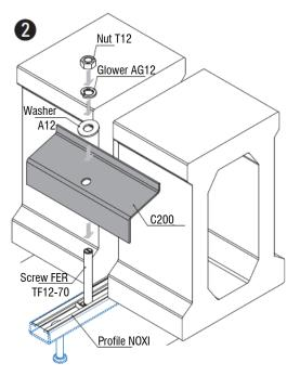
2.1.- Assembly of the screw and the anchor through the hole  $\emptyset$ 13, leaving the shorter wing of the anchor in contact with the beam.
