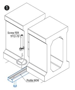
1.1.- Place the FER screw into profile and turn it 90 degrees.
