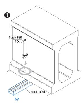
1.1.- Place the FER screw into profile and turn it 90 degrees.
