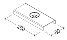
Anchorage for anti-rolling continuous concrete joists placed on a prefabricated concrete structural element. Assembled with C10-60 threaded coupler, VR10 threaded bar, M10 washer, M10 Glower washer and M10 nut.
