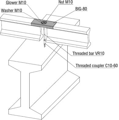
2.1.- Final checking of process. Nut strongly tightened.
