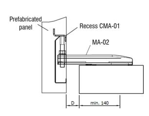
4.1.- Assembly of precast concrete panel.
