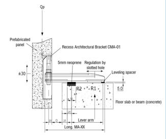
Surface treatment:Hot-dip galvanizedService load:See table on backsideCantilever (D):Up to 80 mm
