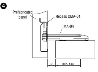
4.1.- Assembly of precast concrete panel.
