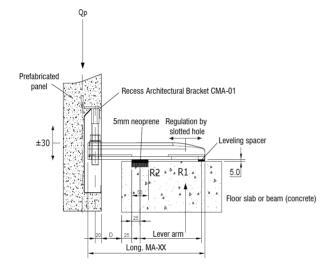
Surface treatment: Hot-dip galvanized Service load: See table on backside Cantilever (D): Up to 80 mm System for supporting panels in architectural permisive. Capacities from 1.242 to 3.457 Kg. Compact design with regulation in the three main directions.
