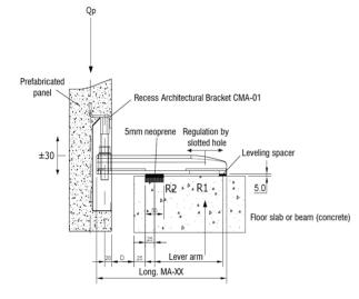
Surface treatment: Hot-dip galvanized Service load: See table on backside Cantilever (D): Up to 150 mm System for supporting panels in architectural permisive. Capacities from 570 to 1.540 Kg. Compact design with regulation in the three main directions.
