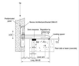
Surface treatment: Hot-dip galvanized Service load: See table on backside Cantilever (D): Up to 80 mm System for supporting panels in architectural permisive. Capacities from 830 to 1.540 Kg. Compact design with regulation in the three main directions.
