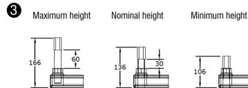
3.1.- Height adjustment through the screw's head. MAXIMUM HEIGHT WILL NOT NEVER EXCEEDED AT ANY CASE.
