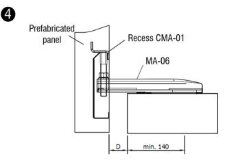
4.1.- Assembly of precast concrete panel.
