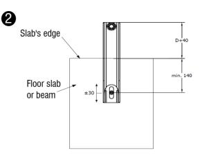
2.1.- Fixing the corbel on concrete slab in order to fulfil nominal position (cantilever measure).
