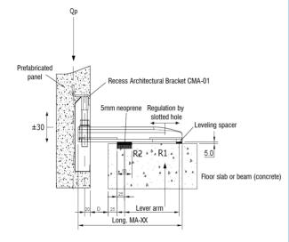
Surface treatment: Hot-dip galvanized Service load: See table on backside Cantilever (D): Up to 130 mm System for supporting panels in architectural permisive. Capacities from 932 to 3.755 Kg. Compact design with regulation in the three main directions.
