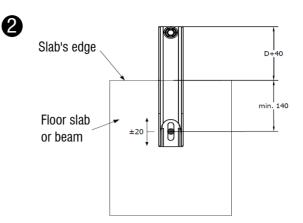
2.1.- Fixing the corbel on concrete slab in order to fulfil nominal position (cantilever measure).
