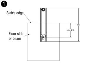
1.1.- Check surface concrete slab where corbel will be placed (plain and clean).
