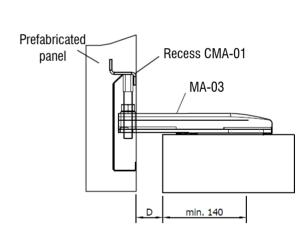
4.1.- Assembly of precast concrete panel.
