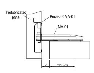
4.1.- Assembly of precast concrete panel.
