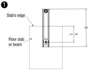
1.1.- Check surface concrete slab where corbel will be placed (plain and clean).
