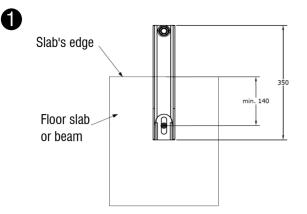
1.1.- Check surface concrete slab where corbel will be placed (plain and clean).
