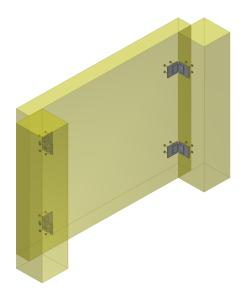
Once the concrete is placed on the support, check that the anchor plate is aligned with the support surface and that there is not any imperfection caused during the assembly phase.
